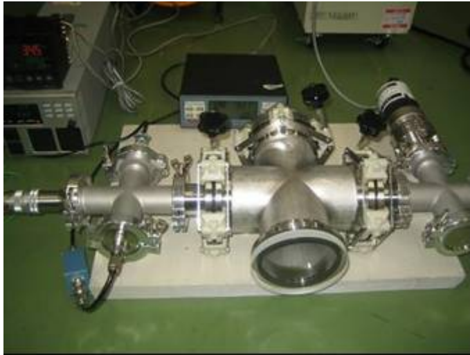
Chamber to make contamination samples.
