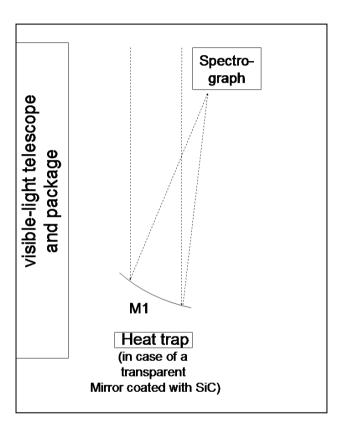
Solution 2: Independent 30 cm quartz mirror coated with 10 nm SiC (or  $B_4C$ ). Due to the lower number of optical surfaces, it yields similar count-rates as Solution 1.
