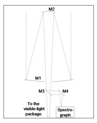
Solution 1: Uses the 50 cm optical telescope (M1, M2 and M4 Al/MgF<sub>2</sub>). M3 is of quartz coated with 10 nm SiC. M4 is used for scanning.
